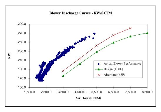
Figure 6 300 HP Centrifugal Blower Curves, Actual and Two Design Conditions (68F and 100F)
