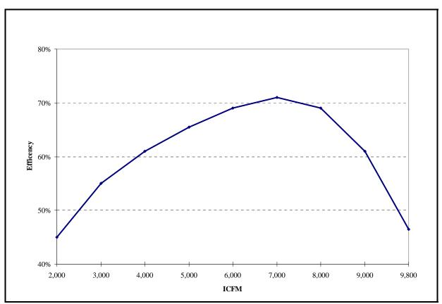
Figure 3 Graph of Mechanical Efficiency of 300 HP Blower
